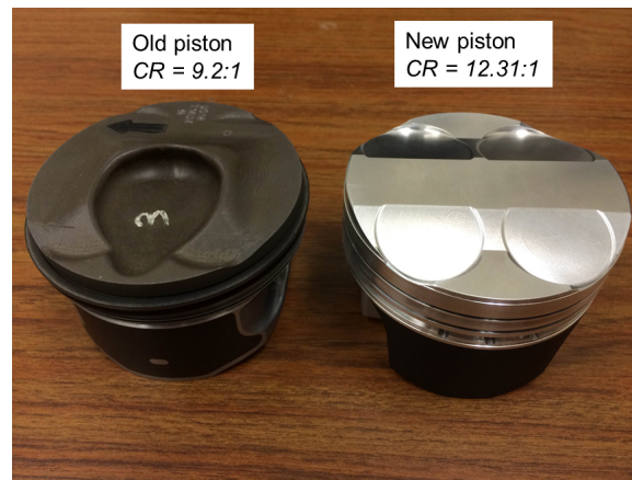
Figure 2.9: Stock and new piston top designs
